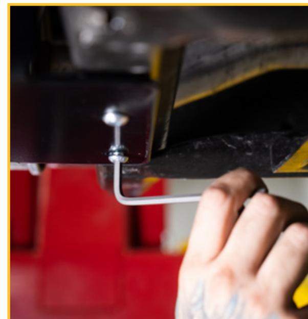
FIGURE 23 (USE BLUE LOCTITE WHEN INSTALLING THE M8 FASTENERS TO THE FACTORY CROSSMEMBER)
