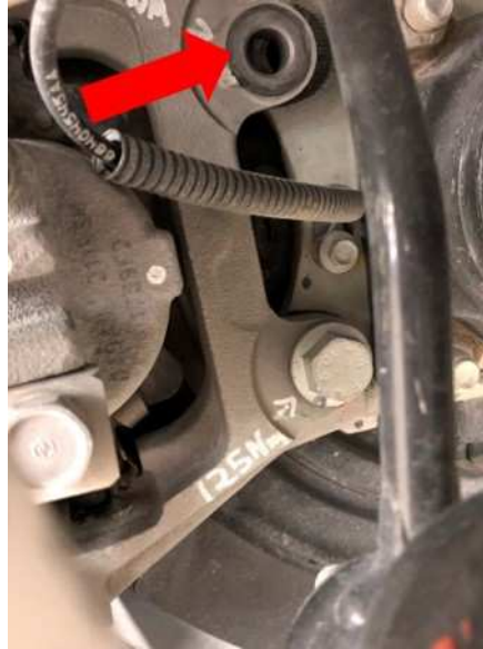
Fig. 1 Missing And Loose Caliper Adapter Bolts
