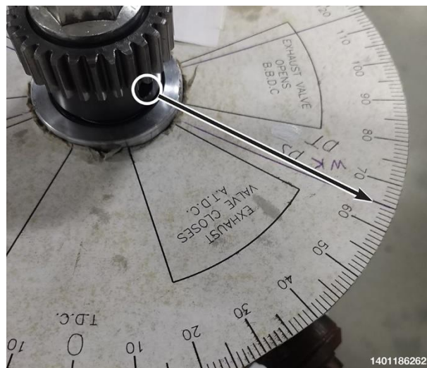
Figure 195 – Installing a Printed Paper Degree Wheel from the Internet
