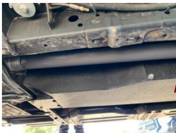
Auxiliary tank installed next to driveshaft
