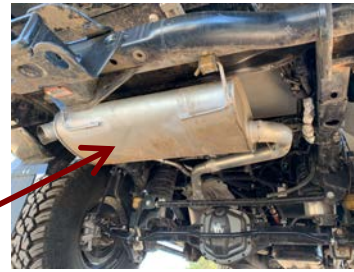
Modified exhaust behind rear axle
