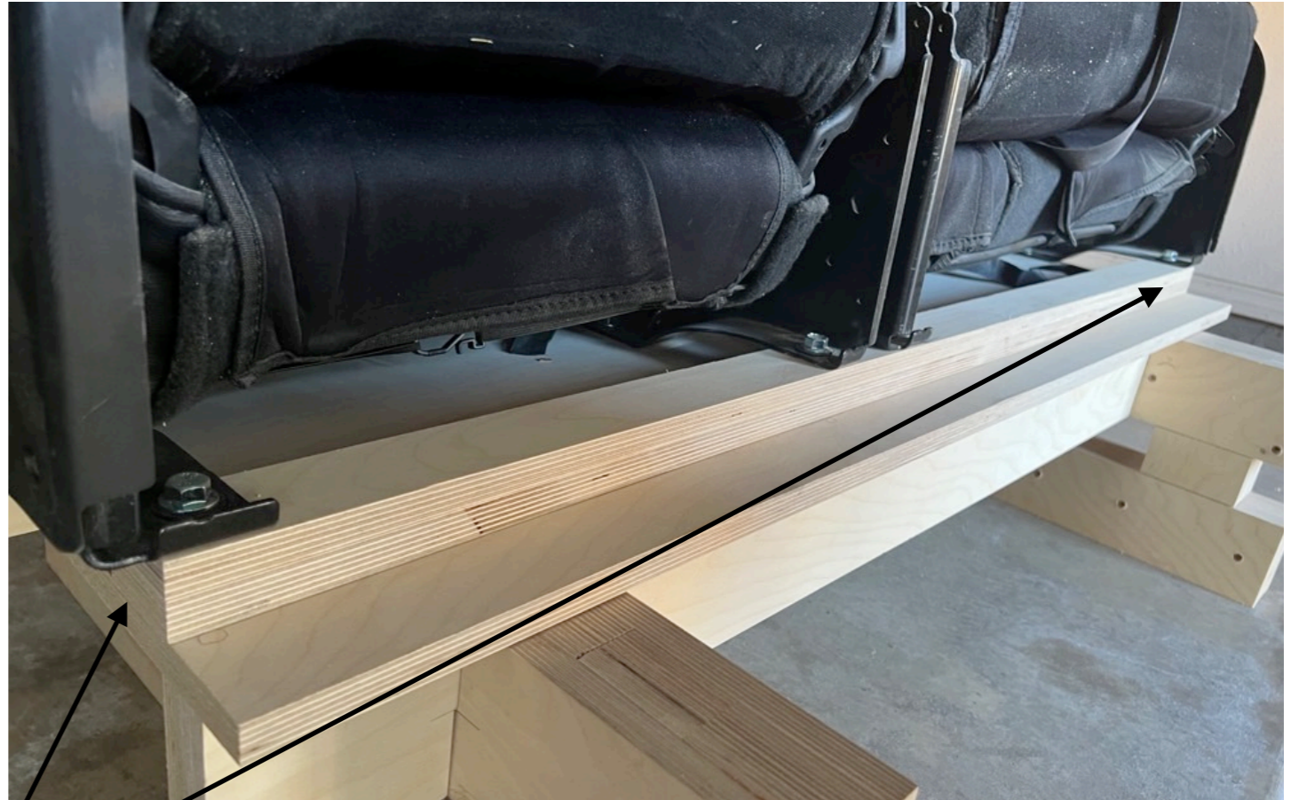
Stretcher bolts on top of platform base
