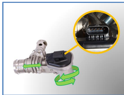
Figure 33: Five-Wire EGR Connector
