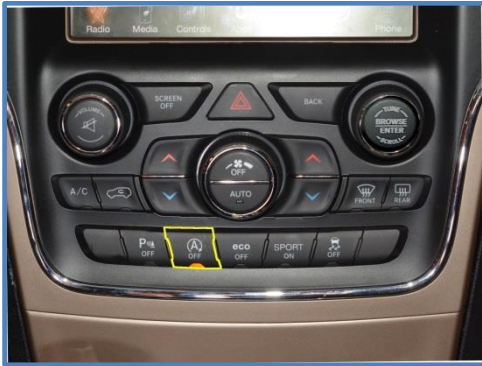
Figure 35: ESS Disable on Center Switch Bank
