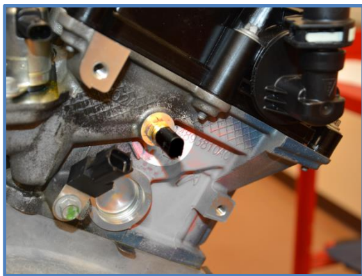
Figure 21: Rear, Right Head Mounted Oil Temperature Sensor
