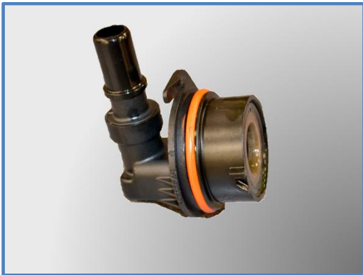
Figure 15: Twist-Off and Quick Disconnect PCV Valve
