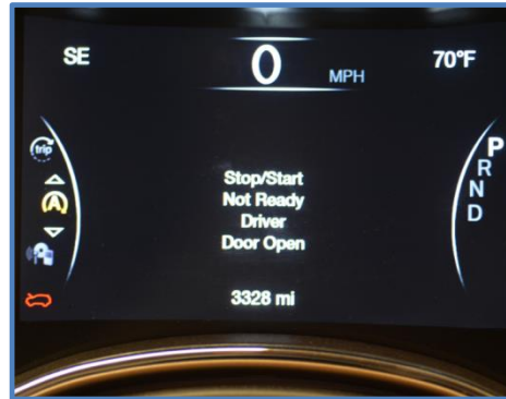
Figure 37: ESS Provides Several EVIC Messages
