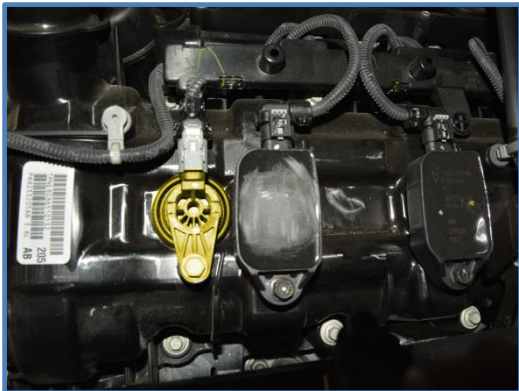
Figure 18: Front VVL Solenoid on Each Bank
