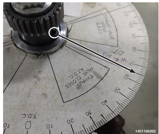
Figure 199 – Installing a Printed Paper Degree Wheel from the Internet
