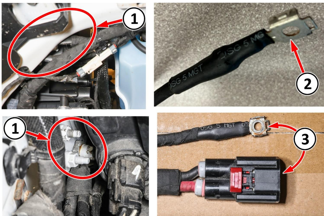
Figure C6 – EHPS ground G908A - Near Left Side Headlamp
