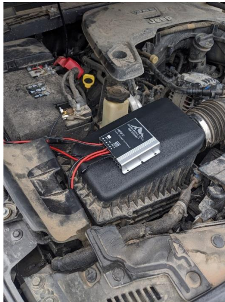
*Above is the preferred mounting location for the charge controller on the air intake box on the Jeep Wrangler JL .
